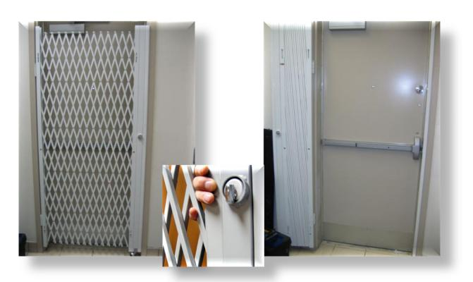
Double diamond webbing and the L206 locking post prevent the hands from accessing the thumb-turn when the security gate is in the locked position.
